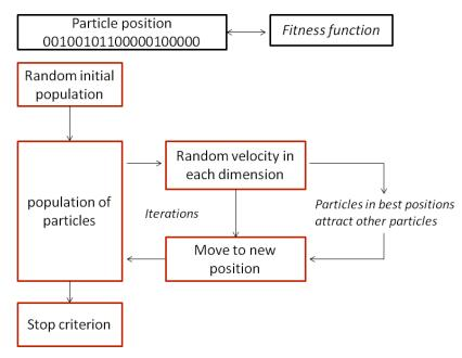
Figure 4. Scheme for PSO algorithm.
