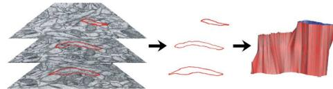
Extracted contours are tiled using the ContourTiler algorithm [BCL'96], incorporated into Volume Rover [CVC].
