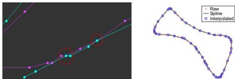
On the left, 2D curation has detected and removed intersections at the indicated locations. On the right, a sample of how splines are used to resample the contours.
