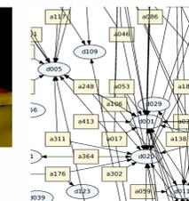
We use synapse data to identify connections between specific axons and dendrites. By collecting this information in a graph structure, we can visualize the wiring connectivity. Merging geometric measurements from the meshes with the graph data will yield a circuit diagram for the entire neuropil volume.
