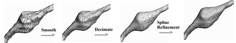
The surface meshes produced by Contour Tiler in the 3D Reconstruction step are often unsuitable for BEMs. We use a suite of tools incorporated into the VolumeRover software package to smooth, decimate, and refine by fitting algebraic splines.
