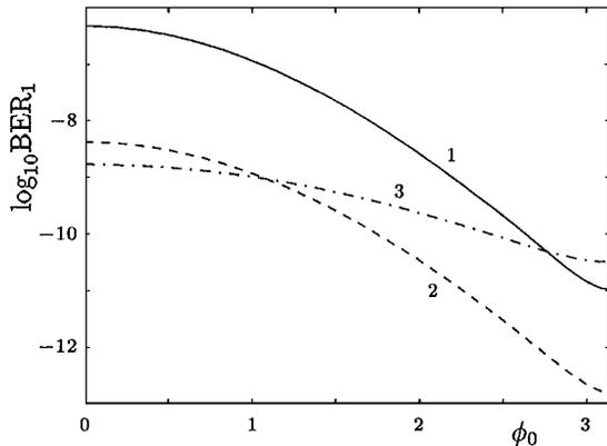
Fig. 4.  $\text{BER}_1$  as a function of initial phase  $\phi_0$ .  $q_0 = 9.5$ ,  $\gamma = 0.4$ ; curve 1,  $D = 0.0003$ ,  $T = 200$ ; curve 2,  $d = 0.0006$ ,  $T = 100$ ; curve 3,  $d = 0.0048$ ,  $T = 25$ .
